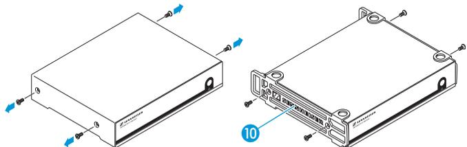
▶ Unscrew and remove the four recessed head screws (M4x8).
