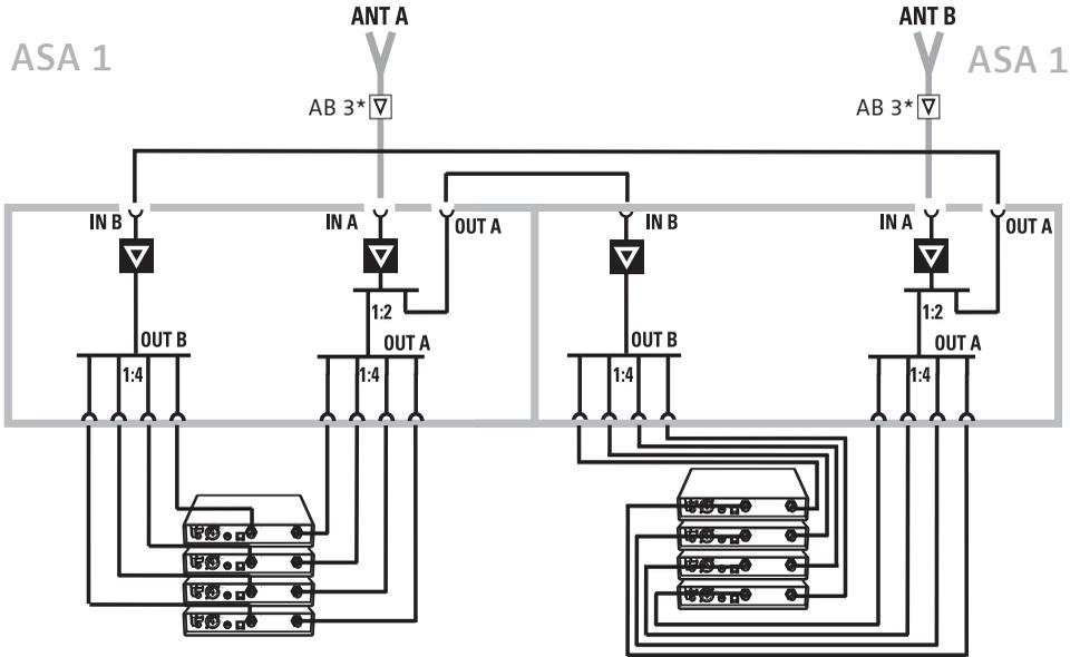
\* AB-3 antenna boosters are only required for longer antenna cables (from approx. 10 m).
