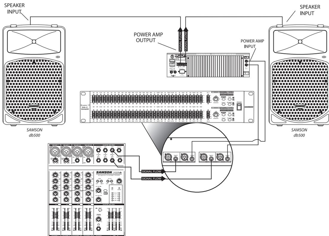
In this example the mixer's stereo output is connected to the S curve 231's inputs. Then, the S curve 231's outputs are connected to the input of a 2-channel power amp. Next, the power amplifier's outputs are connected to the passive (non-powered) loudspeakers.
