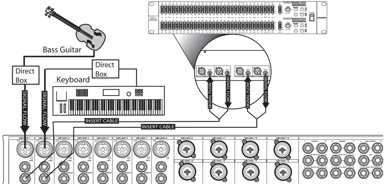
You can use the S curve 231 in your mixer's insert points if you want to equalize two mono channels individually in the mix. In this example the S curve 231's Channel 1 INPUT and OUTPUT are inserted on a bass guitar channel using a 1/4-inch TRS to 2 x 1/4-inch TS "Y" cable, and the Channel 2 INPUT and OUTPUT are inserted on a keyboard channel using the same type of cable. For more information on cable wiring see the S curve 231 Wiring Guide page 15 in this manual.
